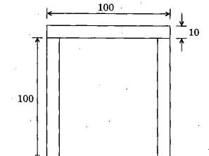
The identical rectangle strips are joined to form a "hat" section. What is the plastic moment capacity?
