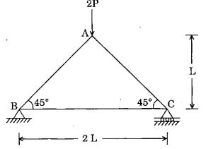
A simple plane truss acted upon by a load 2P at the apex A is shown. The axial force in the member AB is
