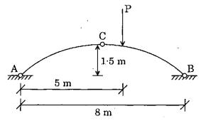
A three-hinged symmetrical arch is loaded as shown in figure. Which one of the following is the magnitude of the correct horizontal thrust?
