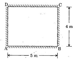
The RC slab, simply supported on all edges as in above figure, is subjected to a total UDL of  $12~\mathrm{kN/m}^2$ . The maximum shear force/unit length along the edge BC is
