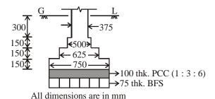
The quantity of BFS under the footing per metre length is
